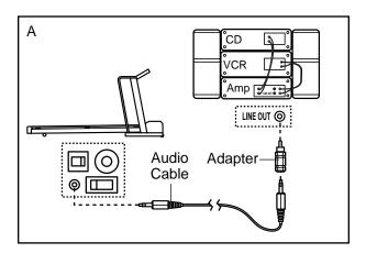
B. Plug one end of the audio cable into the jack on the front of the treadmill near the power cord. Plug the other end of the cable into the included adapter. Plug the adapter into an RCA Y-adapter (available at electronics stores). Next, remove the wire that is currently plugged into the LINE OUT jack on your stereo and plug the wire into the unused side of the Y-adapter. Plug the Y-adapter into the LINE OUT jack on your stereo.
